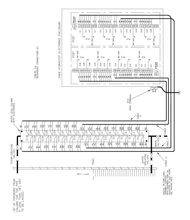
Figure 2.12 - Electrode cable connections to 30 port column
